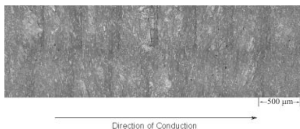
Figure 3 Through-plane thermal conductivity sample containing 65 wt % Thermocarb TC-300 synthetic graphite particles and 5 wt % Fortafil 243 carbon fibers in Vectra A950RX LCP at a magnification of 200 \times .
